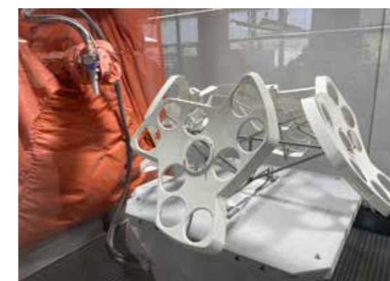
Simple programming Thanks to the 3D CAD programming of the robot, components like this can usually be converted for automatic processing in less than one working day
